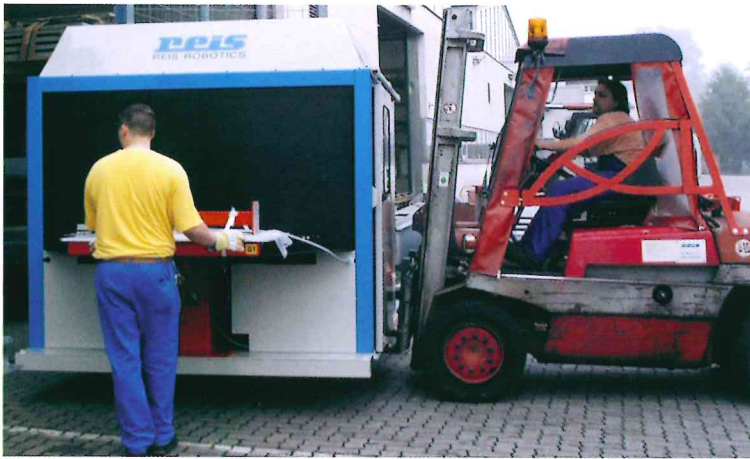
▲ Completely movable welding cabin with 3 ton fork lift truck. Dimensions designed for truck or container transportation.
