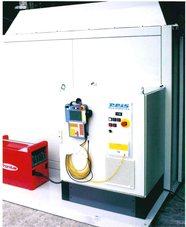
▲ Robot control and weld power source safeguarded from rear, mounted onto continuous base frames. Central media connection.
